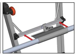
Slide the rung bracket onto the top outer rung as shown above. The rung bracket should sit at 90 degree angle as shown in the image below.
