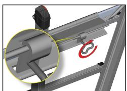
Swing the clamp around and hook it into the open slot in the rung bracket, then tighten the clamp onto the rung. If the clamp will not reach the slot, loosen the clamp all the way, and then try again. Make sure the WingSpan<sup>TM</sup> is secure before each use.
